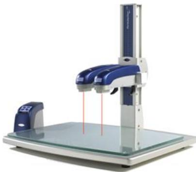
The Formulation Horus ASII is used for analysis of ink drying, the single wavelength laser is shone onto the ink surface to create a speckle pattern. As particles and solvent in the ink move the speckle pattern changes, the change is monitored and the rate of change recorded as fluidity factor. As the ink dries the movement decreases and fluidity factor decreases with distinctive changes at various points from wet to touch dry to full dry.
